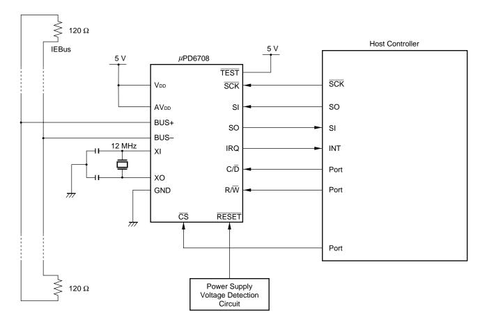
Caution If the power supply voltage moves out of the 5 V  $\pm$ 5 % range, the RESET pin must be driven low for 6  $\mu$ s or more in order to reset the  $\mu$ PD6708.
