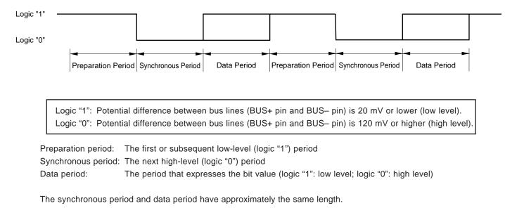
The IEBus uses bit-by-bit synchronization. The specifications for the total bit time and the periods allocated to the bits depend on the type of transfer bit, and on whether the unit is the master unit or the slave unit.
