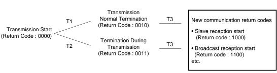
Figure 6-2. Return Code Generation Order in Slave Transmission
